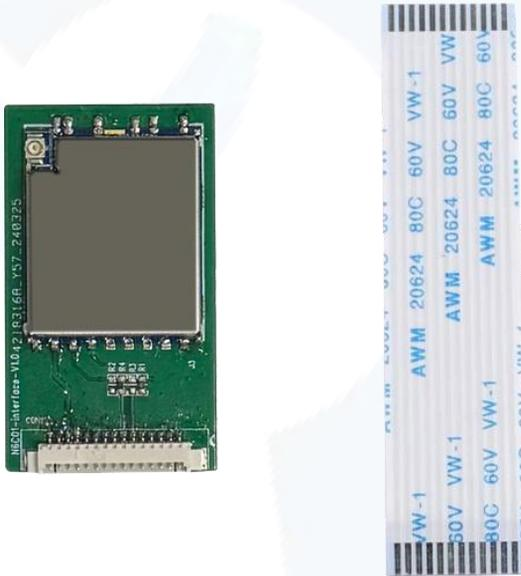
UHF RF module is a high-performance, highly integrated RFID reader IC that integrates functions such as an analog RF front end and a baseband digital signal processing module. Users only need to provide power and communication interface, through the API function library control module work, while the module provides a rich I/O interface, to achieve peripheral device control. Excellent performance can be suitable for various application scenarios
